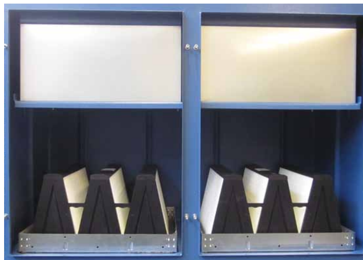
Photo above: Oil mist filter type OUK is also available with additional filter steps through HEPA-absolute filter (above). Compact filter visible below.
