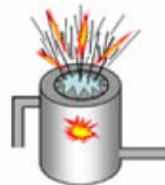
Relief: By membrane or flame-free Hörbiger-valve
