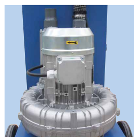
Side channel blower Mounted on vibration absorbers and connected by flex-connections to filter cabinet.
